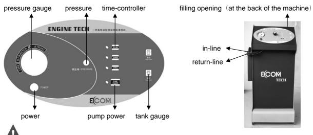
Reference: when the fuel is in low level, the light will be on and alarm.
